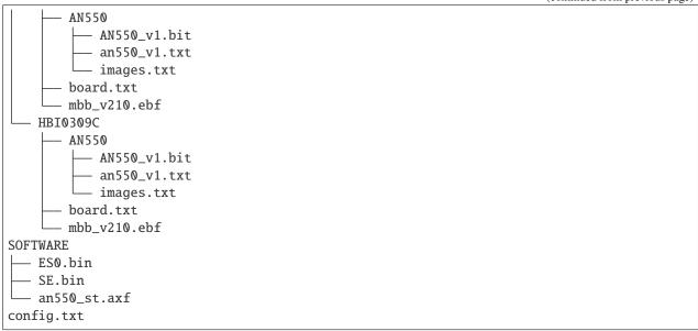
Depending upon the MPS3 board version (printed on the MPS3 board HBI0309B or HBI0309C) you should update the ./AN550/images.txt file so that the file points to the images under SOFTWARE directory.
